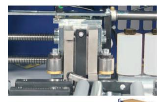
The end trimmer cuts the protruding edges flush to the workpiece at the beginning and the end of the workpiece.
