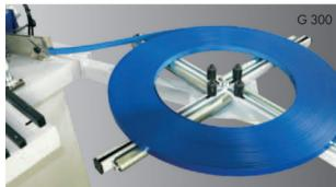
Support for coiled edge material of 0.4 to 2 mm (3 mm for the G 300) incl. rollers and stops.
