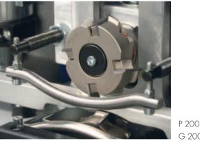
Depending on the setting, the protruding edge is trimmed flush to the workpiece with two cutters on the upper and lower edge of the workpiece and the finish is executed either with a 2 mm radius or 15° bevel cutter. The P 200 and G 200 are equipped with a copying pad, the G 300 with a copy roller.
