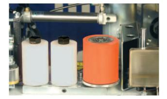
A large rubber-lined contact roller and two plastic pressure rollers ensure that the glue is applied perfectly and the bond well executed.
