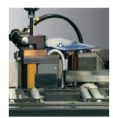
The knurled glue roller ensures an even application of glue to the workpiece. The 1.2 kg glue pot provides sufficient glue capacity.
