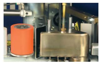
3000 W high performance hot air blower. Variable temperature control 20°–500°C. Temperature display on the thermometer.
