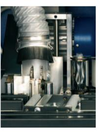
High precision guidance ensure perfect results from the saw unit. The end trimming saw unit guarantees that the ABS edging materials will not discolour once cut.
